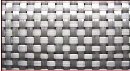
**Figure 1.1 Woven Roving E-Glass Fabric - FGI 1854**
