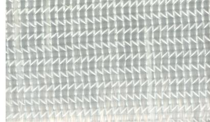
**Figure 1.2 Stitch Bonded E-Glass Fabric - FGI 1800 A2**
